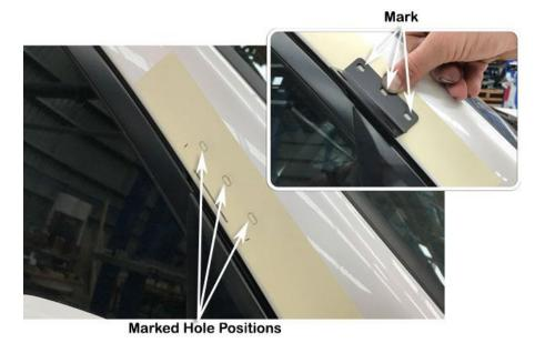
Drill each pilot hole to 8mm diameter with a step drill or 8mm drill bit.
