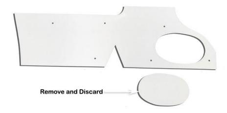
Align the guard panel template (Item 16) to the upper and rear edges of the right hand guard panel as shown.
