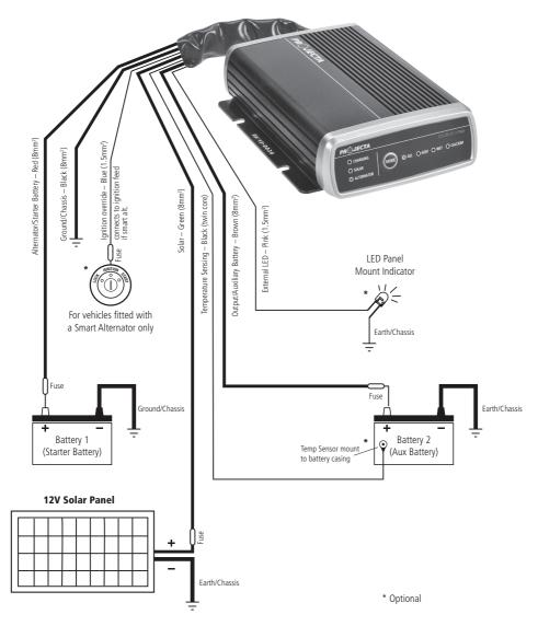
**Important:** For 24V vehicles, a battery master switch is required to connect a 12V solar panel to the IDC45 solar input. This switch is used to turn the solar panel on and off. When solar power is too low to provide fast charge to the auxiliary battery, by turning off the 12V solar panel, IDC45 can provide fast charge through alternator input.
