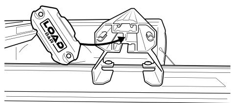
Fasten into position using M4x20mm button head screw.
