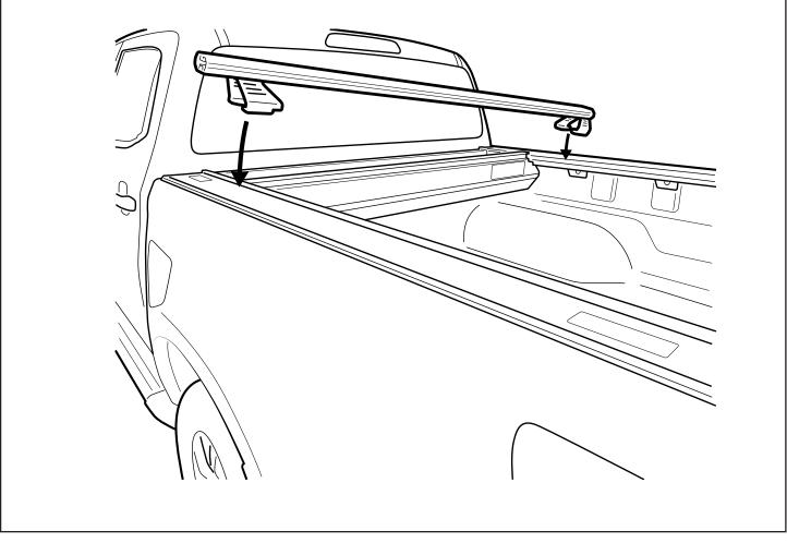
As a guide align cross bar leg center to center of front and rear clamp positions of the roll r cover.
