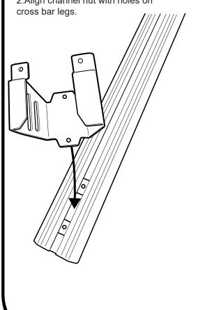
Fasten loosely into place using M6 x 12mm hex bolt and M6 spring washer.
