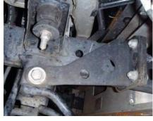
This is the mount from a Genuine Bull Bar. This mount strap uses the bolt hole (below the shock mount) that is required by the tow point. It also conceals the third hole required for correct tow point mounting.
