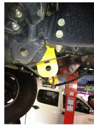
**Ensure all supplied and specified components are used during the installation of tow recovery points, Failure to do so will significantly reduce the Working Load Limit (WLL) specified for each individual point, which can result in serious injury or death.**
