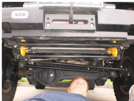
**Ensure all supplied and specified components are used during the installation of tow recovery points, Failure to do so will significantly reduce the Working Load Limit (WLL) specified for each individual point, which can result in serious injury or death.**
