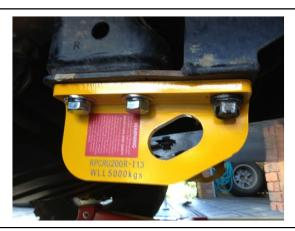
Hardware supplied with RP-CRU200 4 x M12 x 1.25 Bolts 4 x M12 x 1.25 Nuts 4 x M12 Flat Washers 4 x M12 Spring Washers
