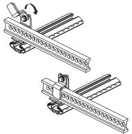
The jack can be secured with a padlock (not supplied) as shown for added security.
