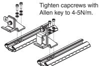
Secure the high lift jack onto the padlock bracket using an M10 x 40 bolt, M10 spring washer and M10 flat washer as shown.
