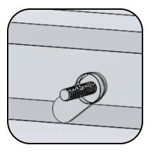
2. Mount RF & RR brackets to underbody of vehicle using supplied nuts, bolts and washers. Make sure nuts and bolts are tightened.
