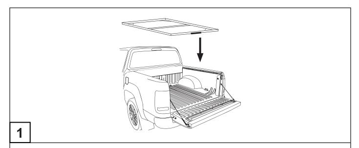
Ensure there is a clearance gap of between 5-10mm from the handle to the tailgate.
