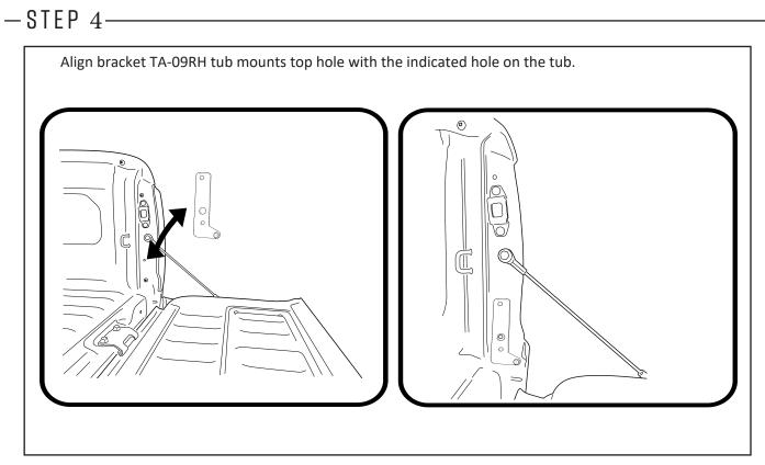
Feed M8 x 20mm button bolt supplied throught the bracket and ute body, fasten using the 3mm thick washer and M8 nyloc nut provided.
