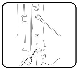
Feed M8 x 20mm button bolt supplied throught the bracket and ute body, fasten using the 3mm washer and M8 nyloc nut provided
