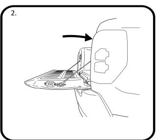
Now repeat all the above steps on the passenger side NOTE: The passenger side Strut has a spacer which will need removing once installed.
