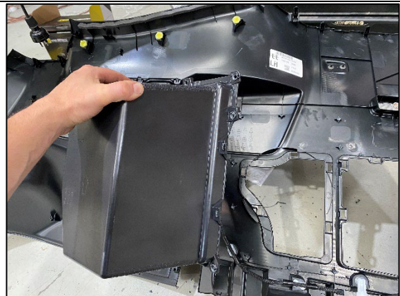
STEP 2.8 PULL FIRMLY ON 2 X RETAINERS ON RHS AND PULL REAR POCKET OFF TO COMPLETELY REMOVE AS SHOWN.
