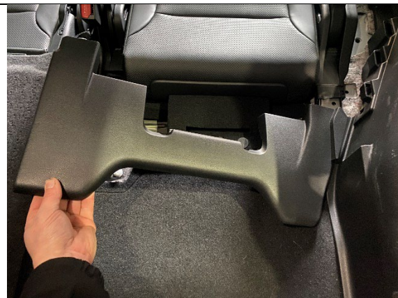
STEP 1.12 MOVE TO THE FRONT OF THE SEAT AND UNCLIP PLASTIC TRIM AS SHOWN (CHECK FOR TRIM CLIPS)
