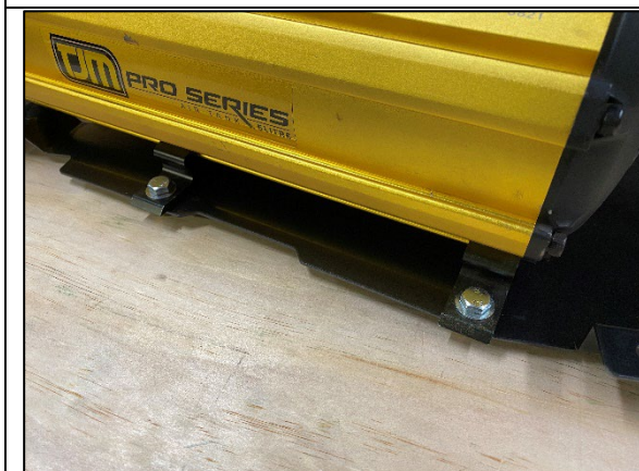
STEP 3.3 FIT TANK TO COMPRESSOR BRACKET USING M8 X 20 BOLTS WITH WASHER UNDER THE HEAD AND FASTEN FROM BEHIND USING ANOTHER WASHER AND M8 NYLOC NUT.
