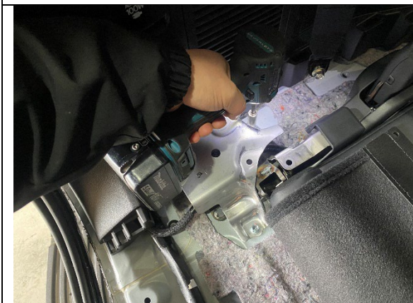
STEP 1.9 REMOVE REAR SUPPORT BRACKETS USING 10MM SOCKET 2 X SCREWS.
