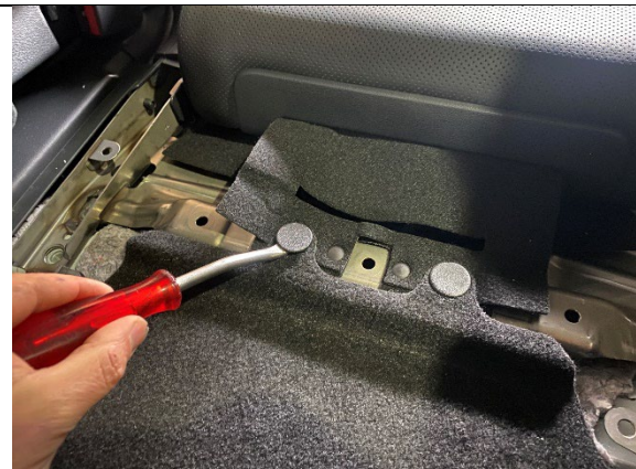
STEP 1.13 PULL OUT THE TRIM CLIPS AS SHOWN. THEY ARE QUITE LONG SO WILL NEED A BIT OF PULLING.
