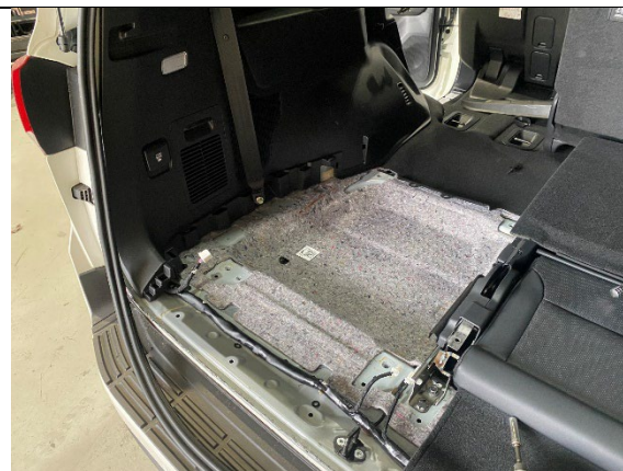
STEP 1.16 PULL THE SEAT OUT AND SET ASIDE AS SHOWN.
