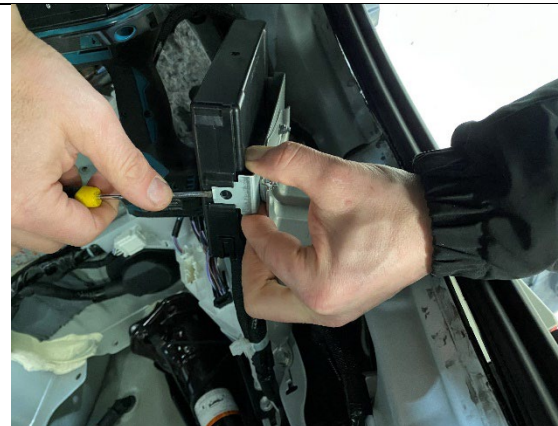
STEP 2.2 USING A SMALL FLAT BLADE SCREW DRIVER, GENTLY REMOVE THE MODULE FROM THE BRACKET AS SHOWN. DISCONNECT WIRING FROM MODULE TP FULLY REMOVE FROM VEHICLE FOR NEXT STEP PREPERATION
