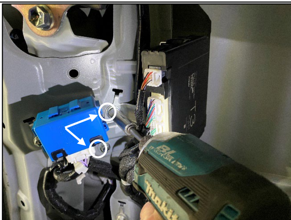
STEP 2.1 REMOVE 3 RD ROW SEAT CONTROL MODULE BRACKET USING 10MM SOCKET X 2
