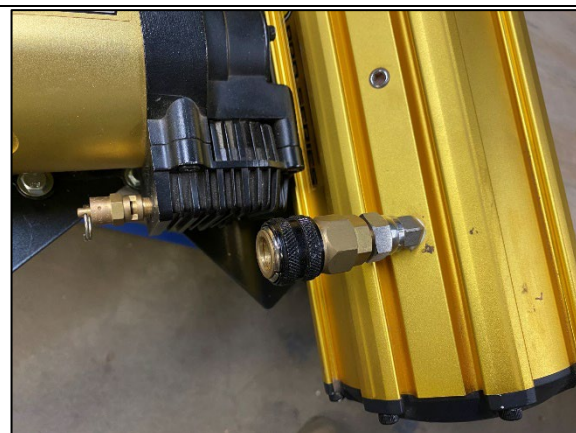
STEP 3.6 FIT THE TJM NITTO FITTING (NOT SUPPLIED) OR JBA-CB112 800MM HOSE IF FITTING AIR OUTLET TO DRAWER FRONT.
