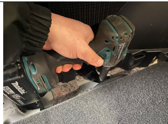
STEP 1.17 REMOVE 3 RD ROW SEAT BELT USING 14MM SOCKET AND RETRACT OUT OF THE WAY.
