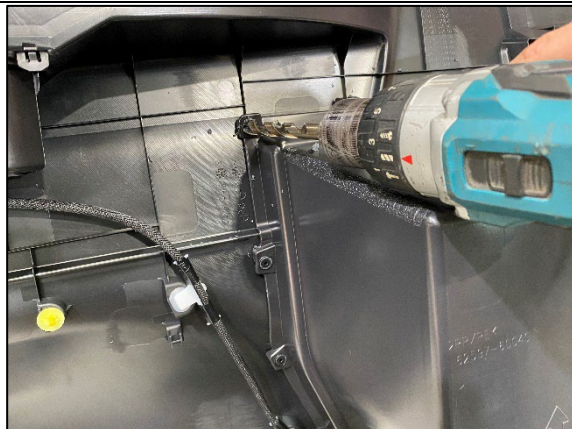
STEP 2.7 USING A 12MM DRILL, GENTLY DRILL OUT THE 9 X PLASTIC LUGS ON THE STORAGE COMPARTMENT AS SHOWN.
