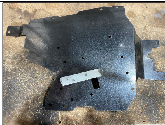
STEP 2.4 MOUNT THE C SHAPED SECTION TO THE BACK OF THE JBA BRACKET USING M4 SCREWS AND NYLOC NUT. ENSURE SCREW HEADS ARE ON TOYOTA BRACKET SIDE AND NUTS ARE ON FRONT SIDE OF JBA BRACKET TO ENSURE CLEARANCE OF SEAT MODULE ON NEXT STEP.
