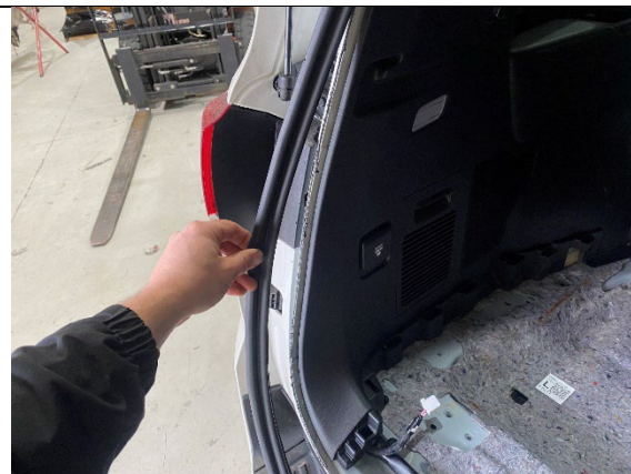
STEP 1.18 PULL BACK THE RUBBER SEAL AT THE REAR.
