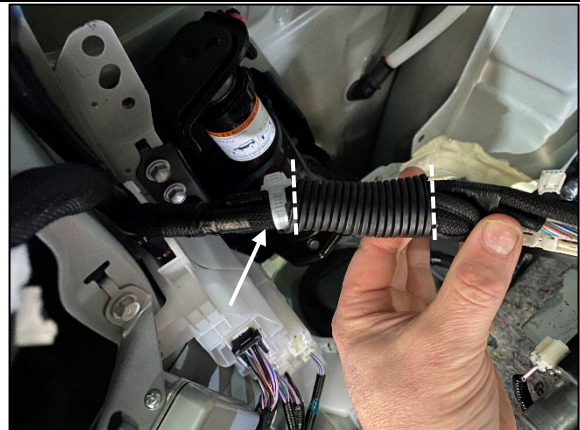
STEP 2.6 SLIDE CONDUIT SECTION OVER TOYOTA LOOM TO THE RIGHT OF THE BODY CABLE TIE CLIP AS SHOWN
