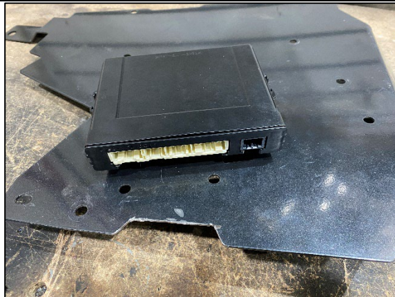
STEP 2.5 REMOUNT ELECTRIC MODULE TO BRACKET AS SHOWN
