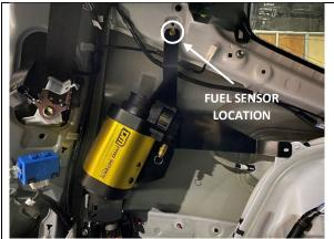
**STEP 3.1** LIFT THE BRACKET INTO PLACE AS SHOWN TAKING NOTE OF THE TOP LEFT FITMENT POINT ALIGNING WITH THE FUEL SENSOR POSITION.
