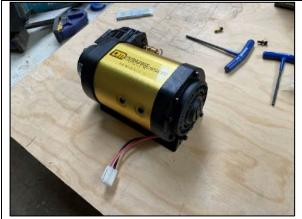
**STEP 2.1** ROTATE THE COMPRESSOR 90 DEGREES ENSURING THE POWER WIRES ARE AT THE BOTTOM OF THE COMPRESOR AS SHOWN.
