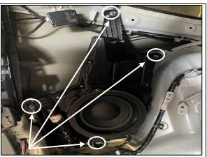
**STEP 2.2** REMOVE THE 4 X M6 SCREWS AND KEEP SPEAKER AND SCREWS ASIDE.
