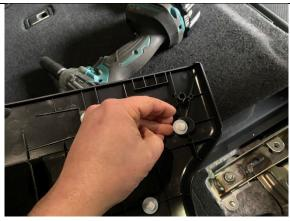
**STEP 1.33** RE-INSERT INTO THE PLASTIC TRIM PANEL LOCATION. THEY WILL NORMALLY SLIDE IN AND POP INTO POSITION. THESE STEPS WILL ENSURE AN EASIER RE-INSTALLATION OF THE PANELS LATER.
