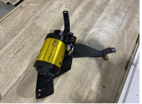
**STEP 2.2** MOUNT COMPRESSOR TO BRACKET IN ORIENTATION AS SHOWN. (THIS PICTURE SHOWN FIRST FOR REFERENCE OF POSITION). REFER TO NEXT STEP FOR NUT AND BOLT ORIENTATIONS.
