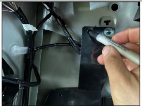
**STEP 1.27** REMOVE FUEL SENSOR ON TOP LEFT AND FIT COMPRESSOR BRACKET IN PLACE LOOSLEY FITTING M6 X 20 SEMS SCREWS. MARK THE TOP LEFT HOLE AS SHOWN AND REMOVE BRACKET.
