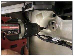
**STEP 1.28** DRILL OUT THE MARKED HOLE TO 7MM AND TREAT EXPOSED EDGES WITH RUST PREVENTATIVE. **BE EXTREMLEY CAREFUL TO ENSURE DRILL BIT DOESN'T PULL THROUGH AND DAMAGE OUTER BODY PANEL.**
