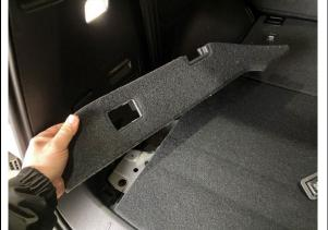
**STEP 1.5** PULL OUT TRIM PANELS (LEFT AND RIGHT SIDES) AS SHOWN. (CHECK FOR ANY TRIM CLIPS THAT MAY HAVE REMAINED IN THE VEHICLE, REMOVE AND REFIT TO THE PANEL SEE STEPS 1.25-1.27).
