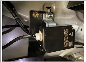
**STEP 3.2** RE-POSITION THE FUEL SENSOR INTO THE BODY T-SLOT AND FASTEN FINGER TIGHT USING SUPPLIED M6 X 20 SEMS ASSEMBLY AS SHOWN. INSTALL SECOND M6 X 16 SEMS INTO PREVIOULSY DRILLED HOLE ON LEFT AND SECURE FROM BEHIND USING M6 WHIZZ NUT.
