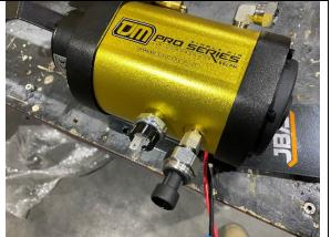
**STEP 2A.4** IF FITTING JBA DIGITAL PSI GAUGE, INSTALL PRESSURE TRANSDUCER TO TOP RIGHT 1/8" OUTLET
