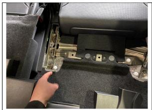
**STEP 1.31** REFERENCE PICS FOR TRIM CLIP (EXAMPLE ONLY). AS YOU ARE REMOVING PANELS, KEEP NOTICE OF ANY CLIPS THAT HAVE REMAINED IN THE VEHICLE- NORMALLY WHITE OR GREEN AS SHOWN.
