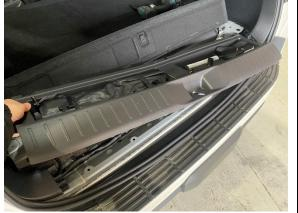
**STEP 1.8** REMOVE REAR TRIM PANEL COMPLETELY AS SHOWN. (CHECK FOR TRIM CLIPS)
