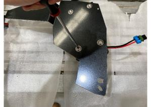
**STEP 2.3** FASTEN FROM REAR OF BRACKET USING M8 DOME HEAD BOLT WITH WASHER UNDER THE HEAD. FASTEN FROM COMPRESSOR SIDE USING WASHER AND NYLOC NUT.
