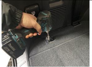
**STEP 1.4** MOVE TO REAR OF THE VEHICLE AND REMOVE TIE DOWN POINTS USING 10MM SOCKET (BOTH LEFT AND RIGHT SIDES).
