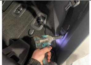
**STEP 1.3** REMOVE THE SECOND ROW SEAT BELT USING 14MM SOCKET.
