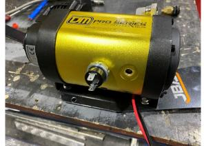
**STEP 2A.3** INSTALL THE PRESSURE SWITCH SUPPLIED WITH TJM COMPRESSOR INTO TOP LEFT 1/8" OUTLET ON THE BOTTOM SIDE.
