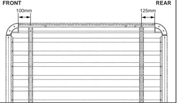
After underbars have been correctly fitted, place the Pioneer Platform on top of the Backbone. Align the underbars with the top tabs and ensure the M8 hardware fits into underbar channel.
