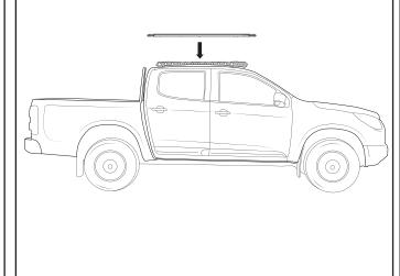
Once Pioneer Underbars have been aligned properly, tighten all M8 hardware using 13mm socket wrench or 13mm spanner. Ensure channel nut has rotated within Pioneer underbar and is fixing Pioneer securely.
