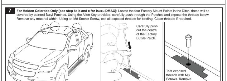
For Isuzu D-MAX: 1 - Measure back along the Ditch from the front of the vehicle, 350mm as shown. Spot drill the centre of the Ditch at this point with a 3mm Drill Bit. Measure back from here a further 1032mm and spot drill at that point. 2 - Open out these spot marks with a 7mm Drill Bit.
