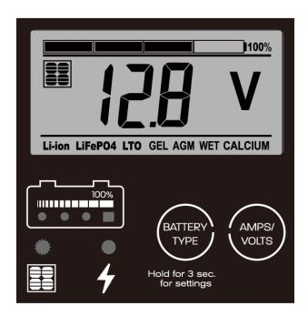
Press **BATTERY TYPE button** and hold for 3 seconds to go into your battery type selection mode. The default setting is AGM Battery; once you select a battery type, the regulator will automatically memorise it for future use.
