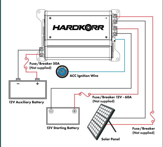
NOTE: First connect the ACC line to the ignition of your vehicle. Then turn your key to the 'ignition on' position. When the engine starts it will be detected by the DC-DC charger and your auxiliary battery will be charged via the main battery.
