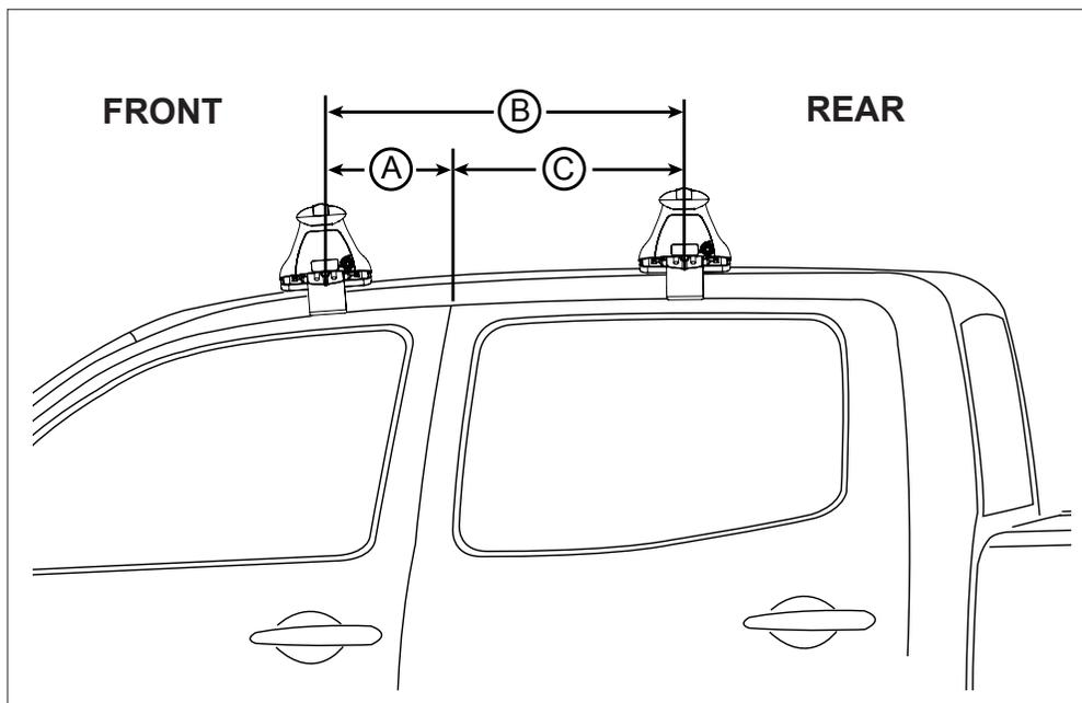
**Note:** Clamps, when placed in position untightened, do not follow the contour of the roof. This will correct as the clamp is tightened.
