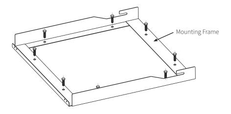
d. Insert the drawer fridge onto the mounting frame. Ensure the locating lugs are securely inserted into the locating slots.
