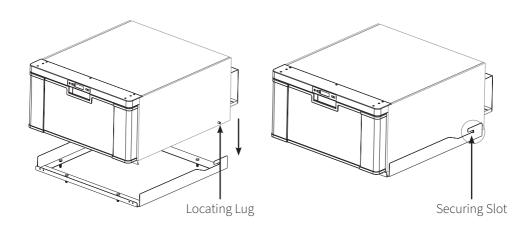
e. Using the 4 screws provided, secure the fridge to the mounting frame as shown below.
