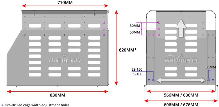
• Pre-Drilled cage height adjustment holes
