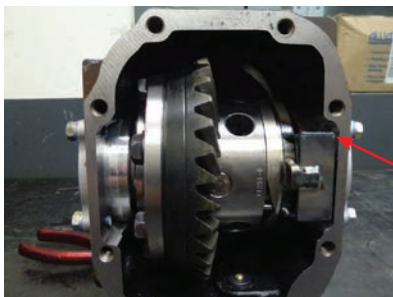
Clearance around the tab
