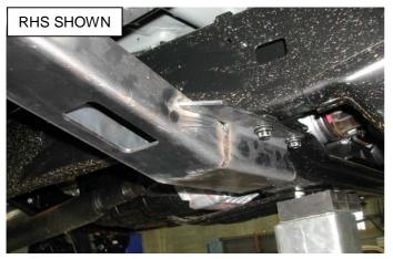
Remove (& discard) the two front fasteners & the outside rear fastener from the gearbox crossmember.
