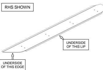
4. Place an end cap plug in the sidebar step end (as shown), then slide the sidebar step end onto the sidebar step sleeve & align the joiner tabs.
