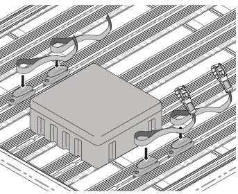
Pull the strap through the Cam Buckle as shown. Tighten over the load to be carried. Ensure load is secure before driving. Tie off any loose ends of the strap.
