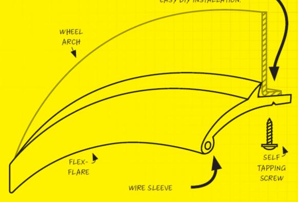
TO INCREASE THE RIGIDITY OF YOUR FLEX-FLARE (AND THE PROTECTION IT PROVIDES), A PRE-FORMED HOLE HAS BEEN EXTRUDED INTO THE SIDE OF THE FLARE, FOR EASY INSERTION OF THE PROVIDED STIFFENING WIRE.
