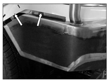
68. Align the FPS so that it is positioned evenly, ensuring that there is a minimum gap of 15mm, between the flare/bumper trim & the FPS.
