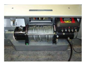
21. If a winch is to be fitted, fit it now following the instructions supplied with the winch.
