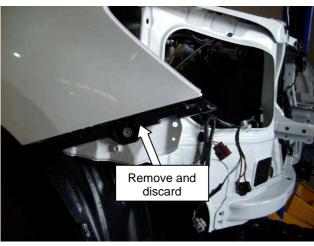
Remove and discard the bumper clips on both side front guards. While the headlights are removed, connect the wiring for the front combination lamps to the vehicles indicator and park light wiring using the scotch locks provided.
