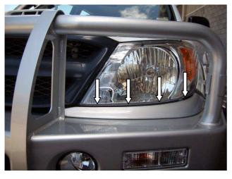
26. If needed, loosen the screws attaching the headlight trim to the bull bar and position the trim so that an even gap is achieved under the headlight. Re-tighten.
