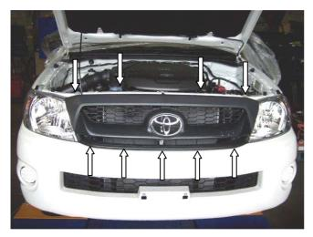
Open the bonnet and remove the two plastic clips and the two screws retaining the top of the grille. From the inside, carefully disengage the clips at the bottom of the grille and remove.
