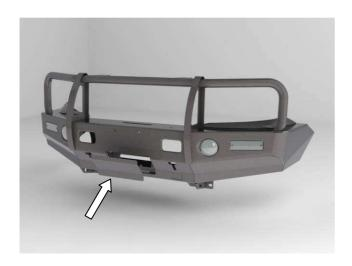
22. If there is to be no winch fitted, fit the winch cover plate to the front of the bar using two M6 x 16mm hex bolts, two ½ x ¾ flat washers and two M6 flange nuts.
