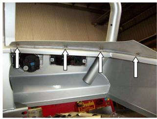
20. Fit the headlight trim to the bar using four 10g x 3/4" screws, flat washers, spring washers and U-nut. Repeat for the opposite side.
