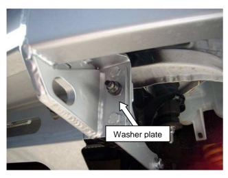
23. With the assistance of another person, carefully lift the bar into position. Attach the bar to the chassis using the washer plate and two of the M10 nuts removed from the intrusion beam. Do not tighten.
