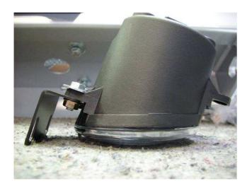
15. Attach the fog light assembly bracket to the fog lights using two M6 x 16mm hex bolts, ½ x ¾ flat washers and M6 flange nuts as shown.
