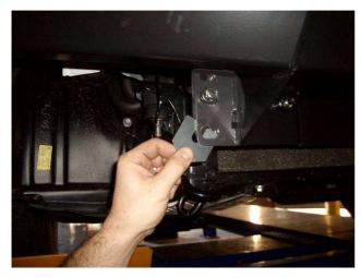
**NOTE:** It may be necessary to position a combination of the supplied shims between the end of the chassis rail and the bar mount, to achieve the required bar position.
