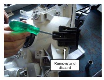
Remove and discard the bumper support clips at the bottom of the headlights.
