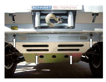
27. To fit the guard to the vehicle, first remove the two bolts that retain the original stone tray. At the top, attach the guard to the two inner studs from the chassis flange. At the bottom, place the guard over the original stone tray and re-insert the original bolts. Using the two remaining M10 nuts from the front intrusion beam and two M10 flat washers secure the guard in place. Tighten all bolts.
