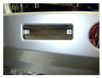
13. Insert nylon plugs supplied into the holes for the indicators and the holes in the front face of the bar for the number plate.
