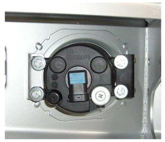
16. Attach the fog light to the bar using two M6 x 16mm hex bolts, ¼ x ¾ flat washers and M6 flange nuts and one fog light washer plate as shown. Repeat for the other side.
