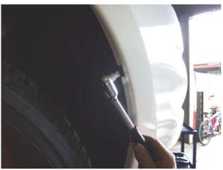
2. Remove the bolts that connect the inner guard to the bumper.
