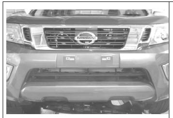
1. Remove number plate mounting block from the front of the bumper & discard.
