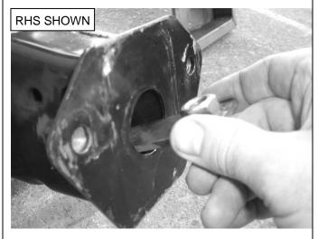
45. Insert the M12 nut-plate (87553) into the right hand chassis rail, through the hole in the chassis rail end plate, & position it over the two holes located in the underside of the chassis rail.
