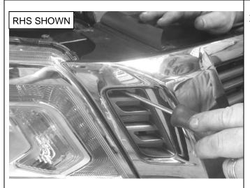
11. Using a flat blade screwdriver, release the four plastic clips (two either side) securing the grille at the front.
