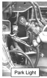
34. Temporarily connect the supplied indicator/park. Check the operation then disconnect.
