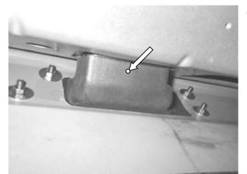
66. Secure the snorkel body to the airbox connector using <sup>3</sup>/<sub>4</sub>" x 8G S/S PK Screw.
