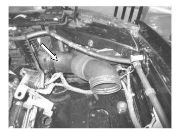
11. Remove and discard the airbox intake tube.
