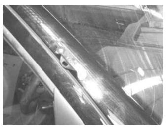
53. Remove the door pillar bracket from the snorkel body (retaining the fastener) and secure the bracket in place on the A pillar, using <sup>3</sup>/<sub>4</sub>" x 8G stainless steel PK screws (2).
