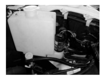
41. Using the washer bottle hose and joiner supplied, connect the pump to the OE washer bottle hose. Re-route the hose and pump wiring from inside the cavity in the inner guard through the side firewall along the wiring harness and to the pump. Use the zip ties (3) supplied to secure the hose in place.
