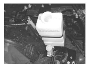
33. Fit the original washer bottle pump retained in step 19, to the washer bottle supplied.
