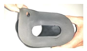
27. Place the intermediate tube foam gasket over the end of the intermediate tube as shown.
