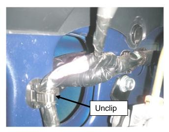
19. From inside the guard, unclip the wire harness from the vehicle and move out of the way to ensure clearance when drilling in step 20.
