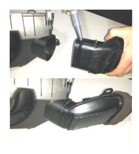
11. Run a bead of neutral cure silicone around the end of the original air box adaptor tube that connects to the air box and refit it back into position ensuring it clips securely. Set aside for refit later.
