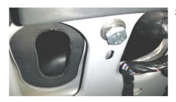
28. Place the intermediate tube in position under the guard and secure with M8x1.25x35mm hex bolt (1), M8 spring washer (1) and M8 flat washer (1).
