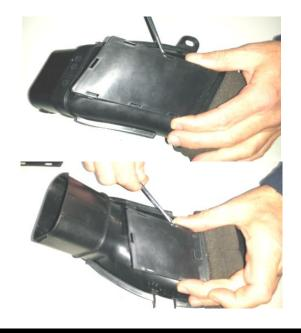
8. Along the sides of the original air box adaptor tube are 2 rectangular covers, one large and one small. Unclip the covers as shown.
