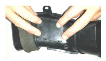
Once the foam gasket is secured in the recess replace the cover. Repeat for the other side.
