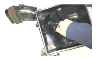
7. Remove the air box adaptor tube from the base of the air box by releasing the clips with a flat head screwdriver as shown.
