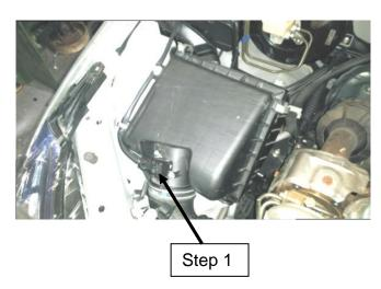
Disconnect the harness connector from the air flow sensor and unclip the harness from the air box lid.
