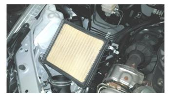
4. Remove and retain the air box lid and air filter element.
