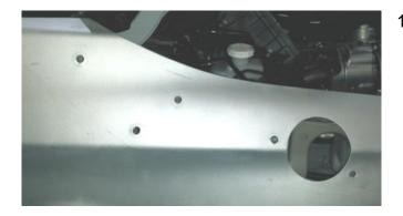
18. Drill the stud pilot holes to 13mm, and drill the snorkel inlet hole to 98mm using a 98mm hole saw.
