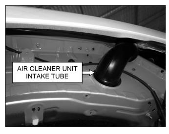
8. Loosen the hose clamp securing the aircleaner unit intake tube to the air-cleaner unit, then discard the air-cleaner unit intake tube (& hose clamp).
