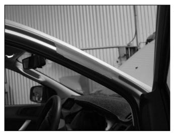
24. To avoid damaging the area when positioning the snorkel body/snorkel bracket, mask the RHS windscreen pillar.
