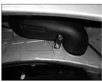
30. Check the clearances between the snorkel body, intermediate tube, air-cleaner unit & vehicle.
