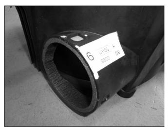
13. Affix the adhesive foam tape to the aircleaner unit base, on the inside of the intake opening (as shown).
