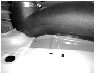
33. Check the clearances between the snorkel body, intermediate tube, air-cleaner unit & vehicle.
