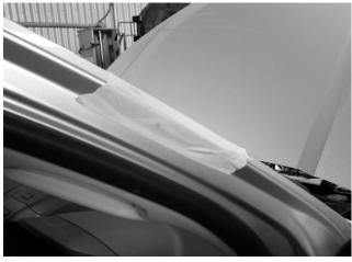
23. To avoid damaging the area when positioning the snorkel body/snorkel bracket, mask the A pillar.
