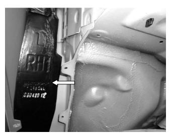
64. Refit the foam fender insert from step 4, as per its original installation.
