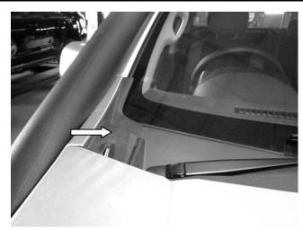
66. Refit the plastic trim moulding from step 5, as per its original installation.
